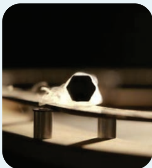
Copper-oxide superconducting pellet levitating over a magnetic track. Courtesy of UBC Science.
