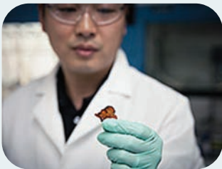
Stanford researcher Chao Wang holds a solid piece of the self-healing polymer used to protect silicon battery electrodes. Courtesy of Brad Plummer/SLAC.
