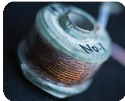
A palm-sized coil is the heart of RAMBO, a Rice-built tabletop system to expose experiments to high magnetic fields. Courtesy of Jeff Fitlow/Rice University.
