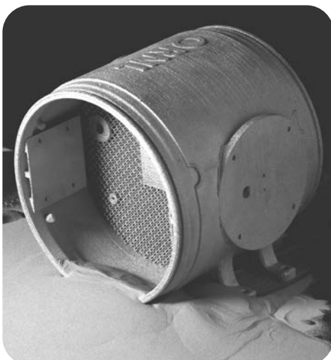
Fig. 3 — Hydraulic manifold built using EBM technology. The part was built at Oak Ridge National Laboratory (ORNL). Courtesy of ORNL.
