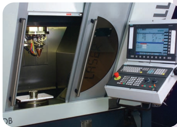
Using laser metal deposition makes the forming die from Mühlhoff Umformtechnik GmbH more robust. Courtesy of Fraunhofer IPT.
