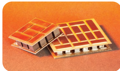
Individual components of thermoelectric modules are only a few millimeters in size. They are cut from specific alloys such as half-Heusler compounds. Courtesy of Fraunhofer IPM.
