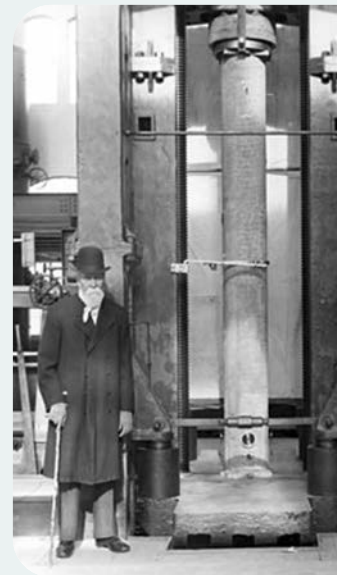
Iron pioneer John Fritz stands beside an 800,000-lb Riehle testing machine, 1909. Courtesy of Lehigh University.
