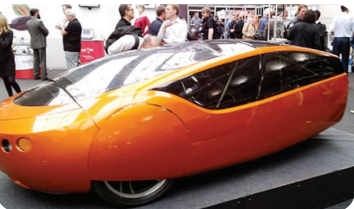
The two-passenger Urbee is the first prototype car ever to have its entire body printed using an additive process.
