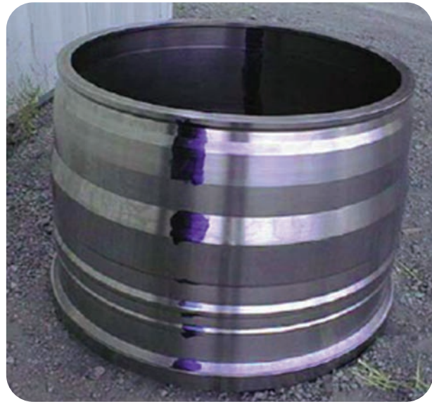
Fig. 5 — Fan case produced by adding features with AM (laser-aided directed energy deposition) to a forged perform. Courtesy of Jim Sears.
