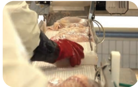
A new machine uses x-rays to locate fish bones then quickly and precisely fillets the fish with a powerful water jet.
