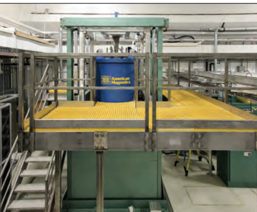
Fig. 1 — ITHMF setup at ORNL consists of a commercial prototype 9-T, 8-in. diameter by 9-in. long uniform field strength superconducting magnet to conduct large-scale experiments.
