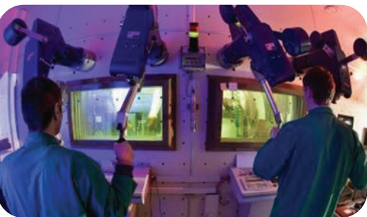
Hot cell testing facility at the Helmholtz-Zentrum Dresden-Rossendorf allows analysis of irradiated material samples.
