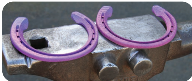
3D printed titanium horseshoes.
