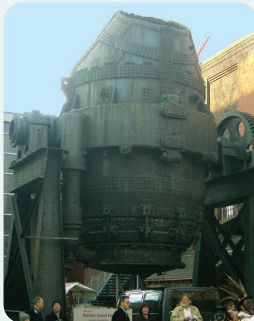
Bessemer converter at Kelham Island Museum, Sheffield, England. Courtesy of Gunnar Larsson.
