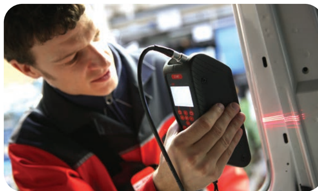
Patented tilt correction leads to reproducible results when evaluating folded edges.
