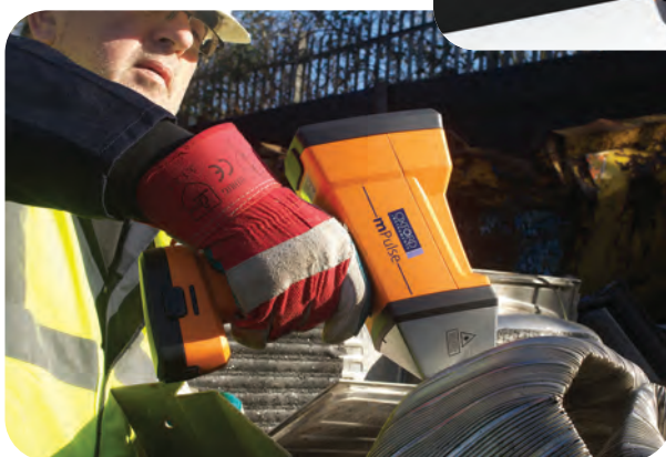
Fig. 1 — mPulse is a handheld portable scrap metal analyzer that enables one-second analysis results used in the field to sort scrap metal.
