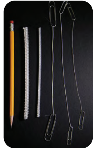
University of Texas at Dallas researchers and international collaborators made artificial muscles in a variety of sizes from polymer fishing line. Courtesy of UT Dallas.
