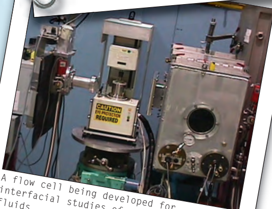
The Couette rheometer sample environment for the 30-m SANS instrument at the NIST Center for Neutron Research.
