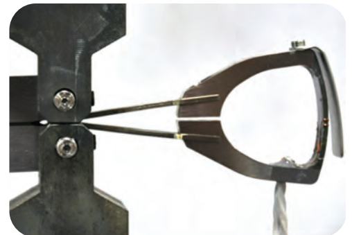
Fig. 3 — Apparatus for the J-R curve test of a compact specimen.
