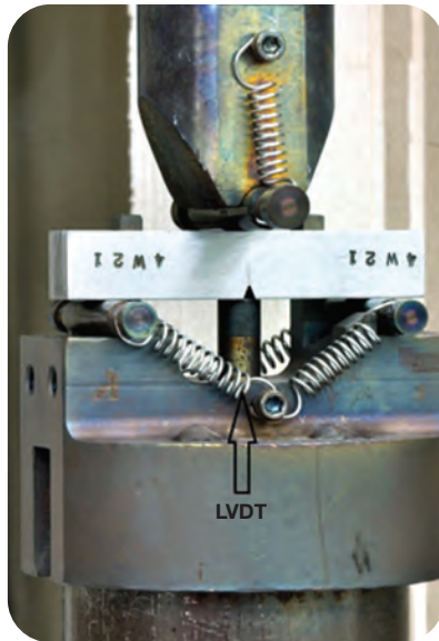
Fig. 4 – Apparatus for the J-R curve test of a single edge bend specimen.
