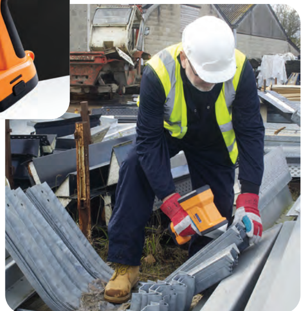
Fig. 2 — The portable mPulse LIBS analyzer allows faster sorting and metal grading.
