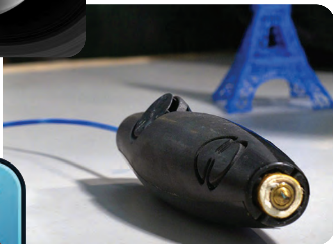
3Doodler is a handheld 3D printing pen that can draw in the air.
