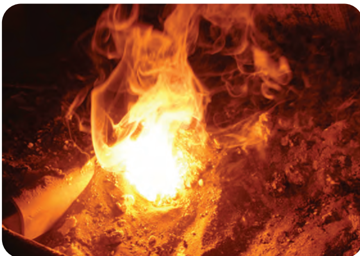
Fig. 1 — Flames of burning Mg-3%Al alloy with extensive fumes and temperature exceeding 3000°C.
