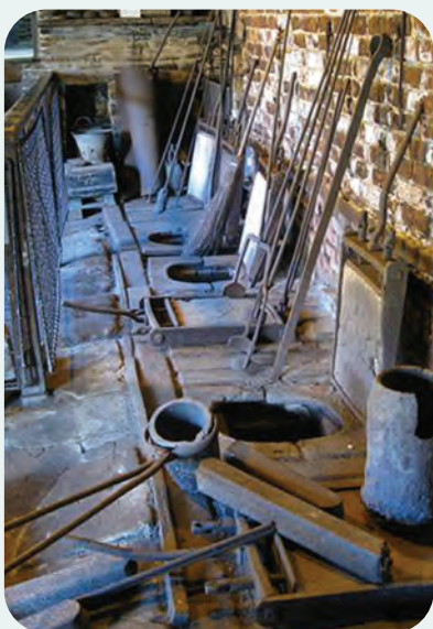
Circa 1829, the crucible furnace at Abbeydale, England, is the oldest example of the type developed by Benjamin Huntsman. Courtesy of www.steelguru.com .
