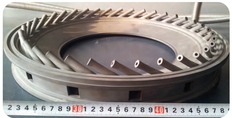
Fig. 5 – A PM net-shape Ti-22Al-24Nb-0.5Mo aerospace engine component.
