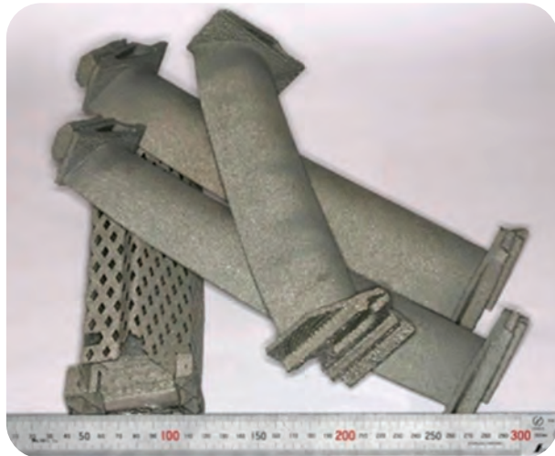
Fig. 6 – \gamma -TiAl LPT blades made by EBM additive manufacturing. Courtesy of Avio S.p.A.
