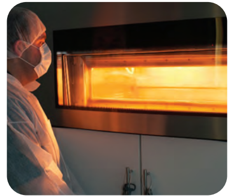
Fig. 3 — Using patient-specific 3D digital data, the cranial implant is additively manufactured with an EOSINT P 800 high-temperature plastic laser-sintering system.
