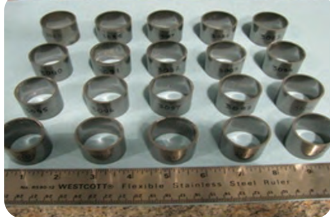
Fig. 7 — Thin-walled (60 mil wall thickness) bonded Nd-Fe-B magnets for automotive and other applications [6] .
