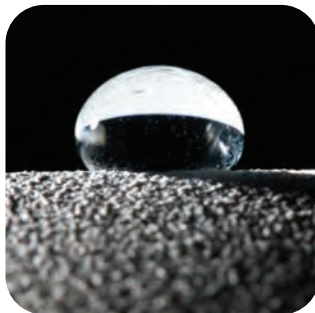
Superhydrophobic surfaces cause water to bead up like a ball. Courtesy of Jaren Wilkey.
