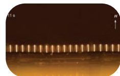
A new material designed by MIT researchers is a flexible polymer skin coated with microhairs (white lines) that tilt in response to a magnetic field. Courtesy of the researchers.
