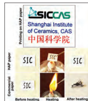
Printing on HAP paper (top). The material is fire resistant (bottom). Courtesy of Ying-Jie Zhu.
