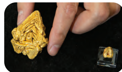
Neutron diffraction data collected on the single-crystal diffraction (SCD) instrument at the Lujan Center, from the Venezuelan gold sample, indicate that the sample is a single crystal.
