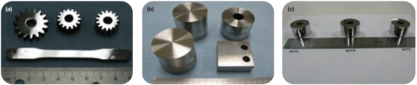
Fig. 5 — CDC compacted and sintered/heat treated advanced stainless steel parts (Custom 465) for naval applications feature wrought-equivalent properties of 250 ksi tensile strength and 17-25% ductility for improved toughness ® .
