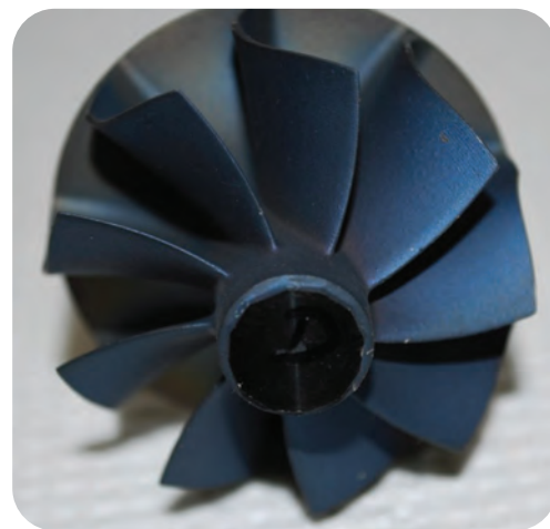
Fig. 1 — Cast 50-mm diameter TiAl automotive turbocharger.
