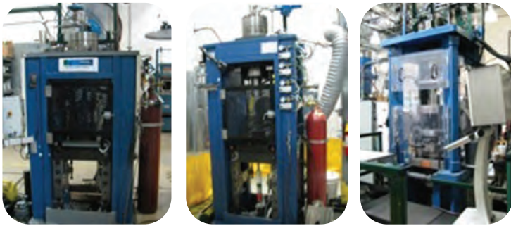
Fig. 2 — Various CDC presses. Left to right: 300-ton manual press, 400-ton manual press, 400-ton automated press.
