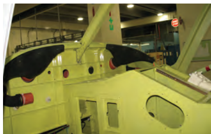
Laser-sintered ductwork installed in a helicopter airframe. Images on this page courtesy of Bell Helicopter Textron Inc.
