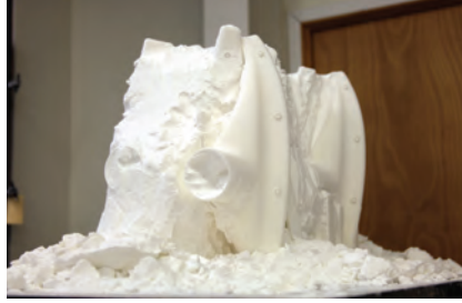
Excess powder is removed and much of it reused for subsequent builds.
