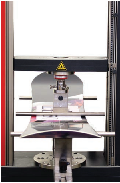
A Nitro snowboard undergoing a 3-point flexural test.
