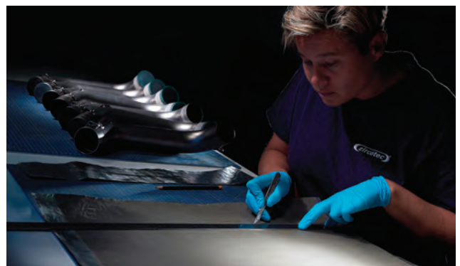
Fig. 2 — ZircoFlex can be cut to shape.
