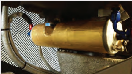
Fig. 5 — JMW Motorsport is using ZircoFlex heat shields to reflect heat away from the transmission's regulator.
