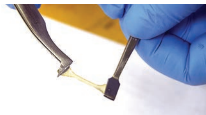
A new kind of self-healing plastic inspired by squid teeth can heal itself with water. Courtesy of Demirel Lab/Penn State.
