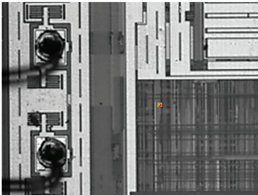
Fig. 4 — Emission microscopy requires little or no sample preparation, other than decapsulation.
