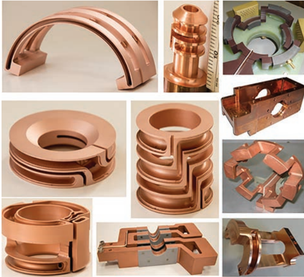
Fig. 2 — Variety of finished and semifinished CNC-machined hardening induction coils.
