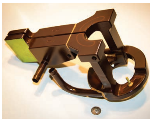
Fig. 5 — Novel inductor design (patent pending) dramatically extends coil life in single-shot hardening of complex shaft-like components.
