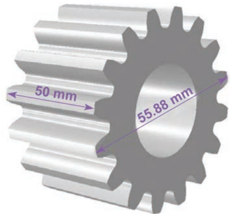
Fig. 1 — CAD model and dimensions of original gear.
