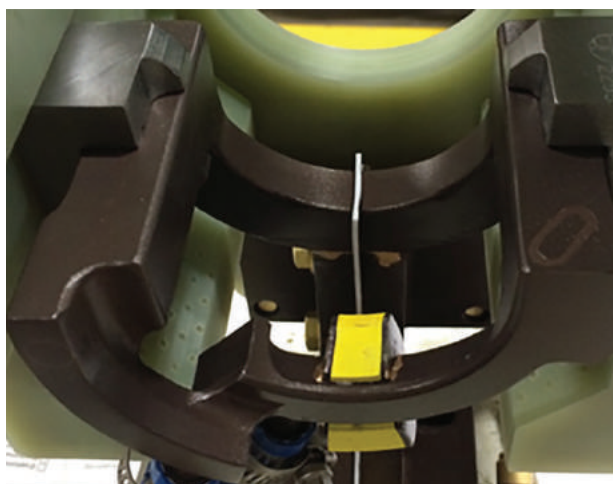
Fig. 4 — A magnetic flux concentrator is attached to certain areas of the hardening inductor coil to enhance localized heat intensity.
