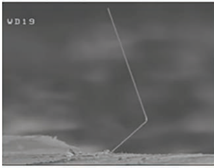
Fig. 1 — Scanning electron microscope image of tin whiskers.
