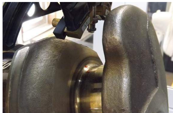
Fig. 5 — State-of-the-art Microarea instrument works in both psi and true chi modes to characterize residual stresses at certain features on a crankshaft without sectioning.
