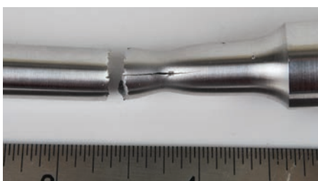
Fig. 10 — Fractured tensile specimen exhibits a longitudinal crack on the bar.
