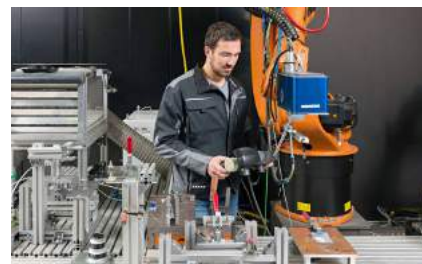
Doctoral candidate André Heckert is working with a laser to fuse plastics with metals. Courtesy of Ulrich Benz/TUM.
