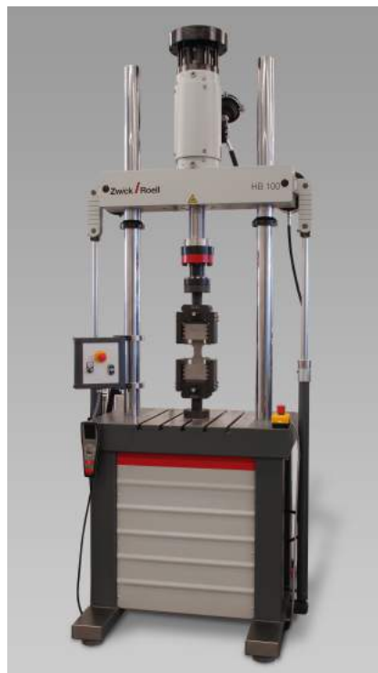
The HB100 servo-hydraulic testing machine has a load range of up to 100 kN.
