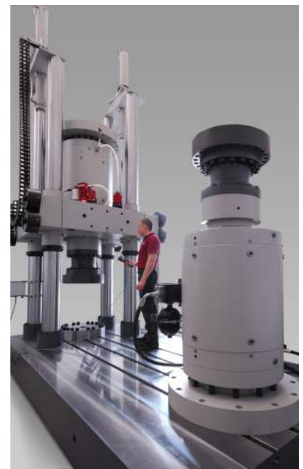
The HB3500 servo-hydraulic testing machine is applicable for testing large components used in construction applications.
