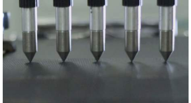
The five-finger scratch test is used to scratch plastics to see how much abuse they can take. Courtesy of Business Wire.
