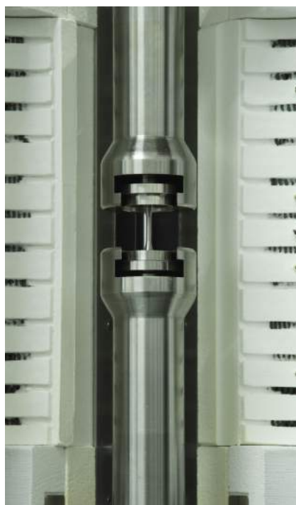
The wide test area of this Vibrophore system accommodates HCF testing at non-ambient temperatures.
