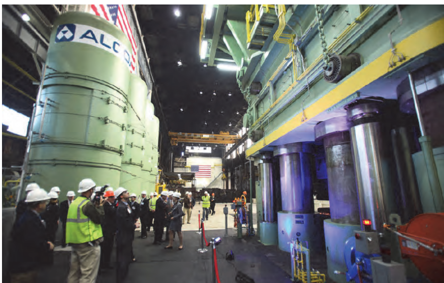
Alcoa's 50,000 ton press, Cleveland, refurbished in 2012.
