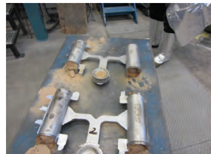
Fig. 5 — Aluminum test components manufactured using strong core technology and high pressure die casting.
