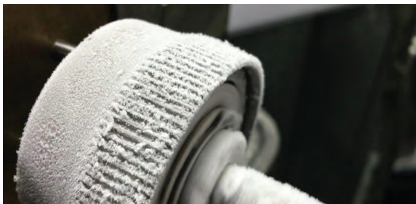
Bulk metallic glass does not become brittle in extreme cold, making it an ideal material for robotics operated in space. Courtesy of NASA/JPL-Caltech.
