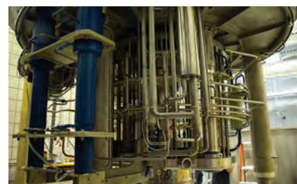
The National MagLab's 33-ton, 36-tesla SCH magnet. Courtesy of Florida State University.
