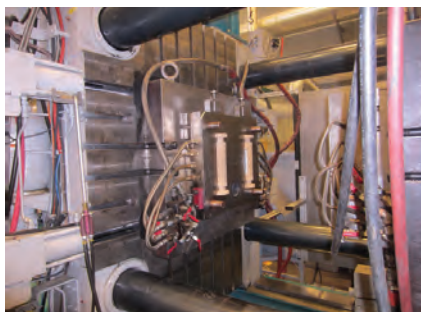
Fig. 4 — Clamp area of high pressure die casting machine with cores installed directly before die closing and injection of liquid alloy.
