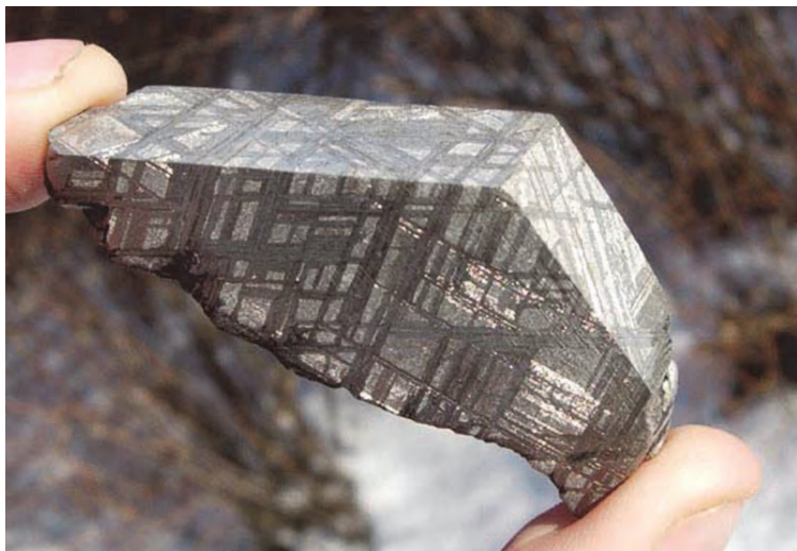
Cross-section of meteorite shows 3D microstructure formed over millions of years.
