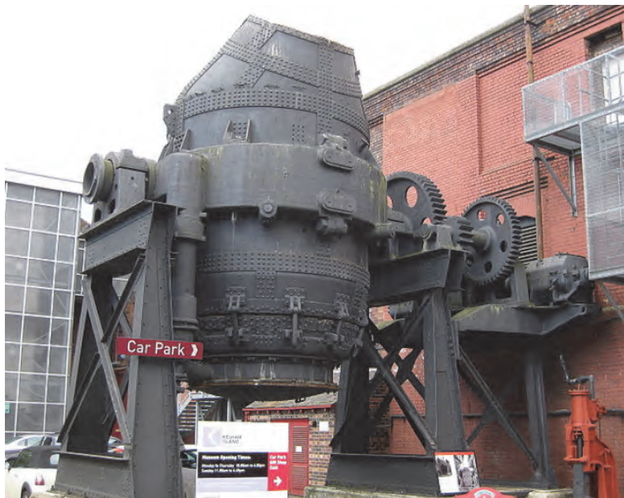
Bessemer converter, Kelham Island Museum, Sheffield, England.
