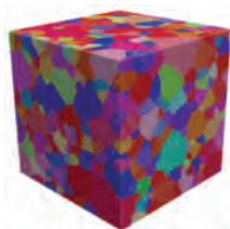
Fig. 2 — Comparison of statistics from a digitally generated tantalum microstructure containing 1500 grains to the real material.
