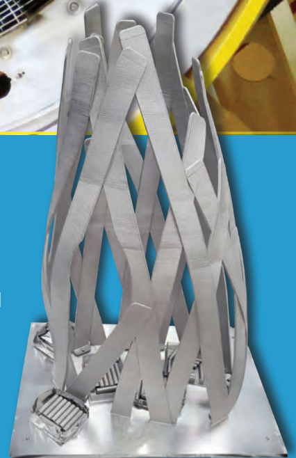
RPM Innovations, Inc. hollow ribbon titanium additive manufactured part vacuum heat treated at Solar Atmospheres (post heat treating)
