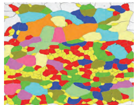
Fig. 5b — Detection of grain interiors by image analysis.
