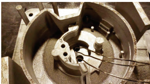
Fig. 5 — AM components often include holes to give thermocouples direct contact with part surfaces, where they can obtain precise temperature measurements.
