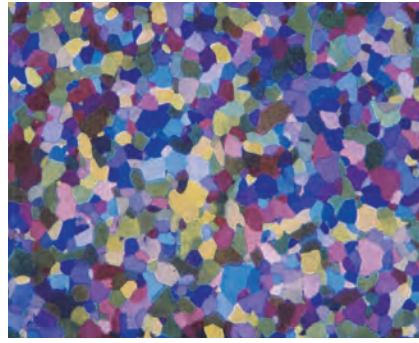
Fig. 1 — Ferrite grain structure of a motor lamination steel etched using Klemm's I reagent at a magnification of 100× (magnification bar removed for grain area measurements).
