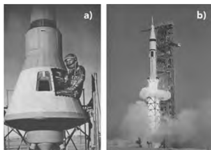
Fig. 2 — (a) Phenolic materials research led to development of the heat shield on the Mercury Spacecraft; (b) high-temperature coatings were also employed on the Saturn 1B launch system.
