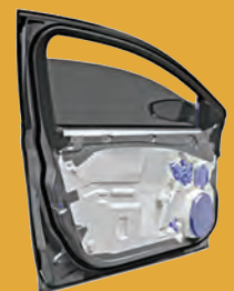
Ultralight door module achieves 42.5% mass savings.
