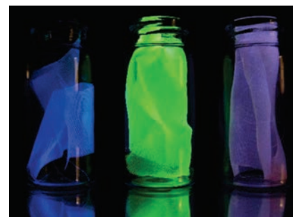
Examples of the silk used in experiments to detect damage in composites, shown under black light. Left, ordinary fibroin of the Bombyx mori silk worm. Observed fluorescence is the result of molecules already present in the fiber’s protein structure. Middle, mechanophore-labeled silk fiber fluoresces in response to damage or stress. Right, control sample without the mechanophore. Courtesy of C. Davis and J. Woodcock/NIST.
