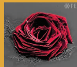
A crystal of cysteine produced by drying a highly concentrated solution of cysteine on a silicon nitride substrate. Courtesy of FEI.
