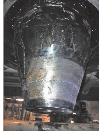
Fig. 2 – Non-coated blow mold head tooling (pin) after 17 months in service.
