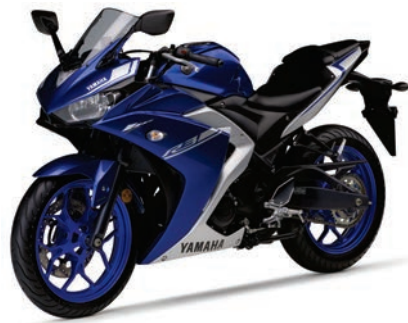
Fig. 2 — Mid-size motorcycle powered by a lightweight 250 cm 3 water-cooled two-cylinder engine. Courtesy of Yamaha Motor Co.
