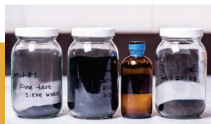
Jars show variations of a patented liquid polymer that looks like water but turns into a ceramic when heated. Courtesy of Kansas State.
