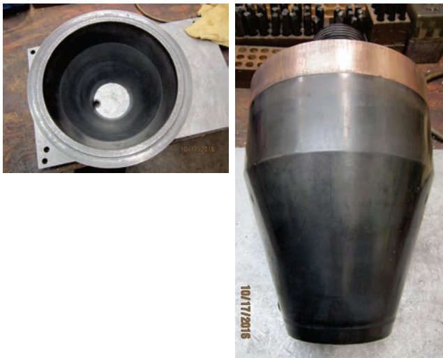
Fig. 1 – Blow mold head tooling (die and pin) coated with a tungsten carbide/cobalt matrix after 19 months in service.
